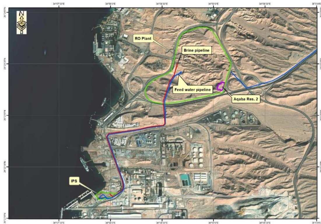
Figure 2-12: Aqaba reservoir 2 at SWRO plant site
